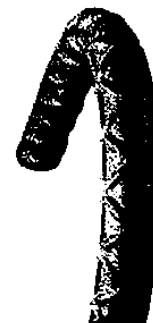
Total damage is nearly 2% of surface area of bar in 1-ft. length, damaged spot is larger than 1/4 in. by 1/4 in., touch-up of damaged spot is required.
