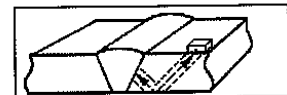
Fig. 5 - Ultrasonic inspection detects discontinuities both on and below the weld surface. Compact, portable equipment makes it easy to use in the field.
